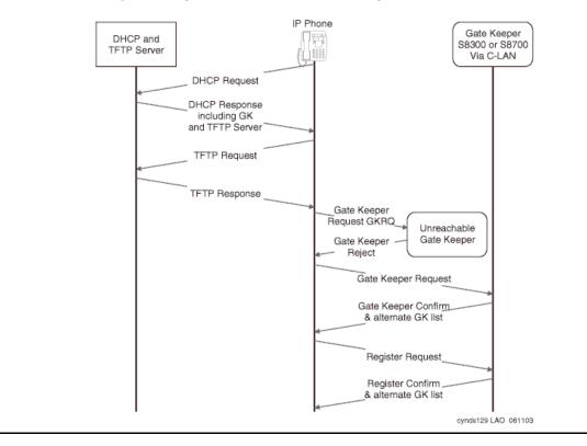
Figure 47: Discovery and registration process to the gatekeeper
